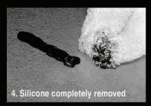
Photos: Dow Corning silicone 791 tested to ASTM C 794-93 specs on galv alum surface.
